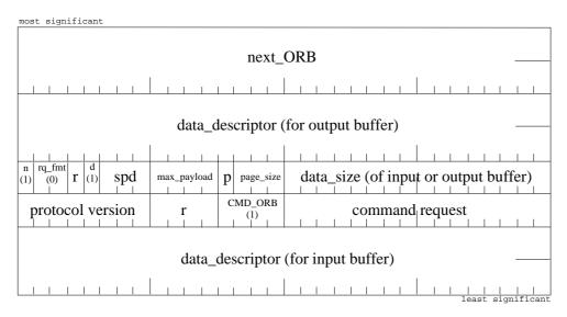
Command ORBs may or may not use an input buffer, and may or may not use an output buffer, depending on the type of command. Most likely the input buffer will point to a ASCII string containing a command in one of several print job languages.
