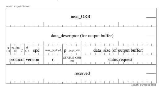
The direction bit, "d", is set to 1 to indicate that the buffer pointed to by data\_descriptor is an output buffer. Note that some status requests use the status block and therefore do not require an output buffer.
