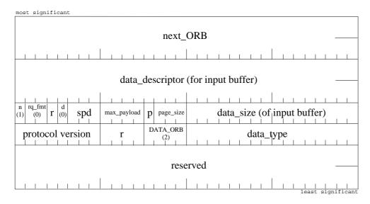
Data\_descriptor points to the buffer containing print data. The data buffer corresponds to SBP-2 specifications. For reference, if "p" (page table) is 0, then data\_descriptor points to the buffer which contains printing data, and data\_size gives the size of this buffer. If p is 1, then data\_descriptor points to the page table, and data\_size gives the number of entries in the page\_table. For a complete explanation, please see the SBP-2 specification.
