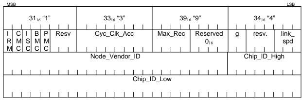
Compliant devices shall implement the bus information block located at a base address offset of FFFF F000 0404<sub>16</sub> in the format defined by this profile.
