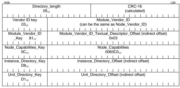
Compliant devices shall implement the root directory located at a fixed address following the bus information block. As shown the root directory is located at a base address offset of FFFF F000  $0414_{16}$ .
