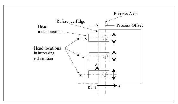
Figure 6 - General Finishing Coordinate System
